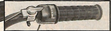
RESPONSIVE CONTROL! Twist-grip throttle on handlebar for positive speed control. Automatically returns to idle when released. Fingertip on-off engine switch.
