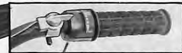
RESPONSIVE CONTROL! Twist-grip throttle on handlebar for positive speed control. Automatically returns to idle when released. Fingertip on-off engine switch.
