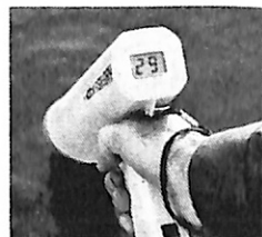
When a fish passes between the Fish Ray and the bottom, depth changes momentarily, telling the fish's depth.
