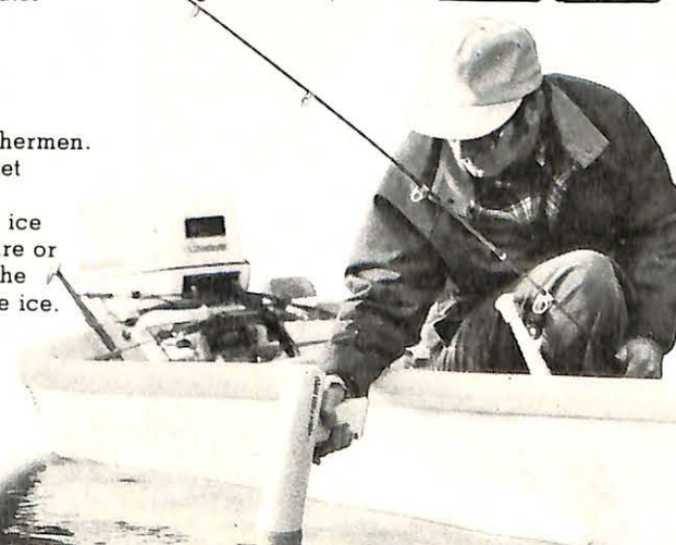
When a fish passes between the Fish Ray and the bottom, depth changes momentarily, telling the fish's depth.
