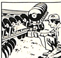
Spray oil on farm machinery as a rust inhibitor or to lubricate hard-to-reach parts.
