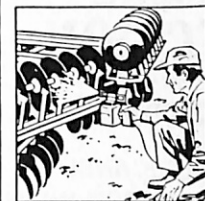
Spray oil on farm machinery as a rust inhibitor or to lubricate hard-to-reach parts.
