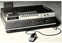
RECORD UP TO FOUR PROGRAMS on four different channels at four different times over a period of 14 days—with the Video Director-Programmable Model VR9700J. Also has Speed Search. Pause/Stop Action and Triple Speed Play features. Cabinet covered with padded chestnut color vinyl leatherette, accented with champagne gold color highlights. Zenith Radio Corp., Public Relations Dept., 1000 Milwaukee Ave., Glenview, IL 60025
