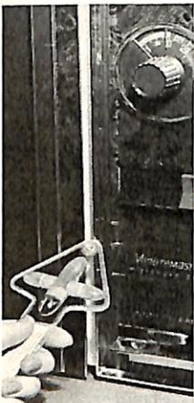
**VEXILAR, INC.** INTRODUCES a low-cost microwave leakage detector. The hand-held device, for use outside the oven, contains a light emitting diode which glows red on contact with microwave radiation in excess of 5 milliwatt, the standard maximum level allowed by the U.S. Food & Drug Administration. Suggested retail cost is under \$20. Vexilar, 9345 Penn Ave. So., Minneapolis, MN 55431
