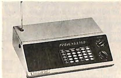
**50-CHANNEL SCANNING MONITOR** tunes in citizens to local happenings. Bearcat 250 scanner uses no crystals, so not knowing exact frequencies no problem. Automatic scanner locks into active channels and radio stores frequencies found in its memory. U.L. Listed and F.C.C. Certified. Available at Bearcat dealers or write Electra Co., 300 E. County Line Rd., South, Cumberland, IN 46229.
