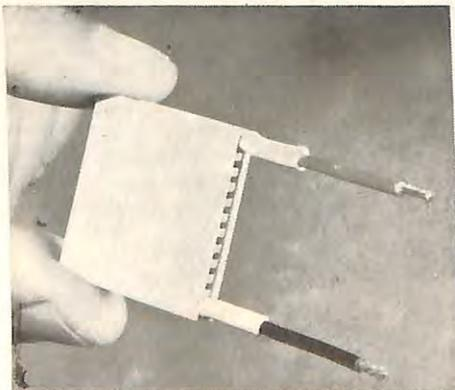
Two of these miniaturized thermoelectric modules replace all the bulky complex piping coils, compressors and motors in conventional portable refrigerators. The modules pump heat from your food into efficient heat sinks where it is dissipated by a quiet fan. They operate on a principal called the "Peltier Effect" - passing electricity through the junction of dissimilar metals causes heat to flow from one metal to the other.
