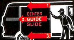
price, a new gliding side door for cargo handling in cramped alleys and beside loading docks. Three separate tracks, at top, bottom and center, give bridge-like support for solid, smooth one-hand operation, tight seal.
