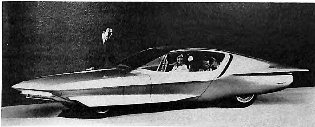
The Firebird IV (top left) has no rear window. Driver receives television views on front panel. The Mako Shark II (right), is an experimental Corvette.
