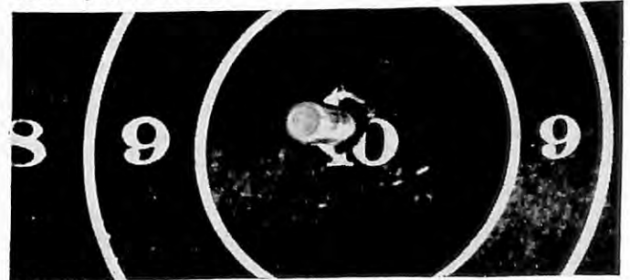
At the target. In this amazing high-speed photograph, a bullet is shown entering the hole made by a previously fired bullet. Now, that's accuracy. The rifle was fired from a machine rest.
