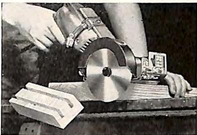
**SUPER SAW** rips and crosscuts up to 2" boards. Arco Saw attaches to any 1/4" electric drill. Dado-Arbor swivels saw-blade to cut grooves up to 1/2" wide x 1" deep in 1 cut. Has graduated gauges for ripping, depth and angle cuts. Model 460. \$12.88 ppd. with blade, instructions. Arco Tools Inc., Dept. EL-11P, 421 W. 203 St., N.Y. 10034.
