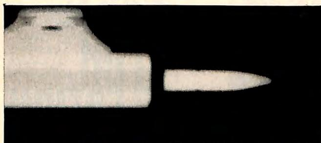
**Leaving the barrel.** The last X ray shows a bullet departing the barrel, being pushed by the hot gases. At this critical point, accuracy is greatly influenced. Slight deflections, yawing or other abnormal conditions at the muzzle can be detected with this X-ray technique, which "sees" through the muzzle blast.
