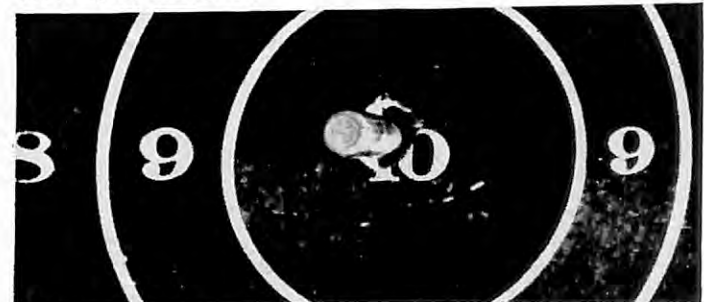
At the target. In this amazing high-speed photograph, a bullet is shown entering the hole made by a previously fired bullet. Now, that's accuracy. The rifle was fired from a machine rest.
