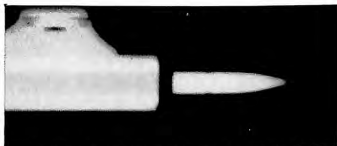
Leaving the barrel. The last X ray shows a bullet departing the barrel, being pushed by the hot gases. At this critical point, accuracy is greatly influenced. Slight deflections, yawing or other abnormal conditions at the muzzle can be detected with this X-ray technique, which "sees" through the muzzle blast.
