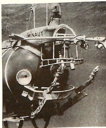
The deep submersible, Aluminaut, shown above gliding through the ocean near Bimini in the Bahamas, has a design depth capability of 15,000 feet—deepest of the research submarines. The 51-foot, aluminum-hulled vessel has taken part in research and salvage operations around the world, often working more than a mile below the surface. Owned and operated by Reynolds Sub-Marine Services, a subsidiary of Reynolds International, Inc., the Aluminaut can carry seven men and more than three tons of scientific equipment and stay submerged for up to three days.
