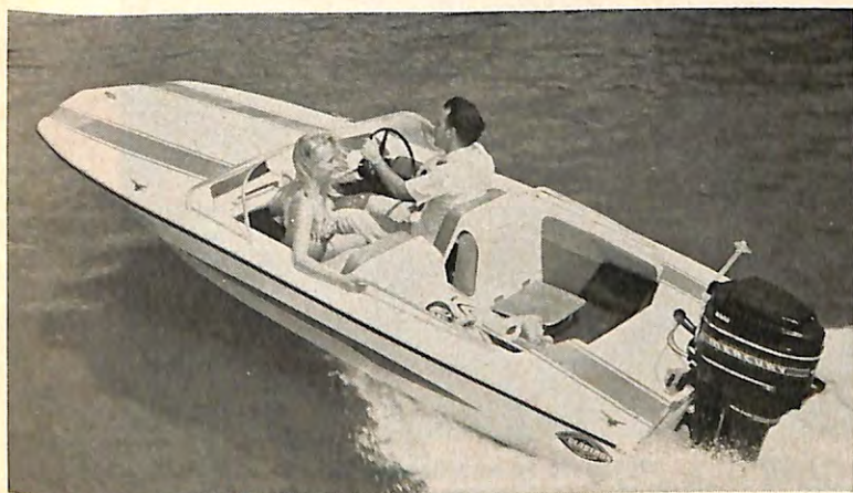
The Glastron V-187 Fundeck (right) is an all-around boat for family use. A 94 inch beam and stern drive power up to 130 H.P. makes skiing easy.
