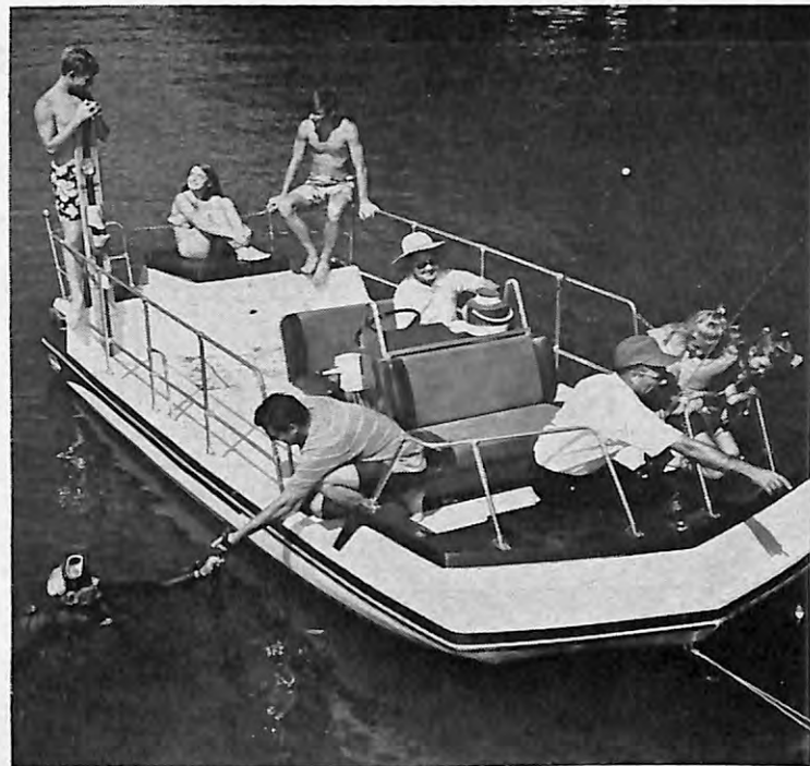
A new big water boat—for inland or offshore use—is offered by Glastron of Austin, Texas. The V-191 (above), 19-foot Sportsman features elevated center console with mechanical steering, letdown windshield, and twin swivel seats.
