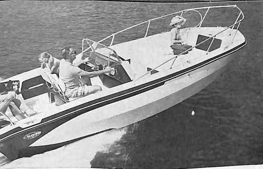
A new big water boat—for inland or offshore use—is offered by Glastron of Austin, Texas. The V-191 (above), 19-foot Sportsman features elevated center console with mechanical steering, letdown windshield, and twin swivel seats.
