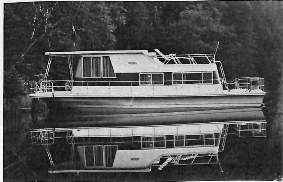
Boatel of Mora, Minnesota announces the 37 ft. fiberglass Cougar (above). This model is carpeted, sleeps 8 and features one-piece hull and one-piece deck, cabin and roof construction. Power comes from a single 250 H.P. inboard/outboard engine.
