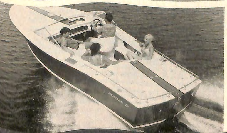
Bertram Yacht of Miami, Florida offers this powerful 20 ft. cruiser (below) in its 1970 line. The all-new 215 H.P. V-8 MerCruiser, stern drive, powering this racy craft is capable of swinging props up to 20 inches in diameter.
