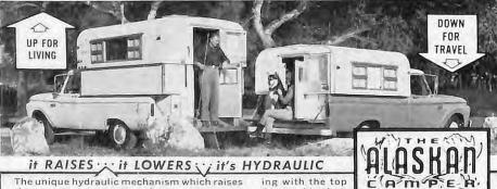
The unique hydraulic mechanism which raises the camper top can be safely operated even by a small child. Locks prevent accidental lowering. The top is lowered quickly by the simple turn of a valve. Drive safely at any speed with minimum drag and sway. Sit or recline on comfortable couches while travel-
