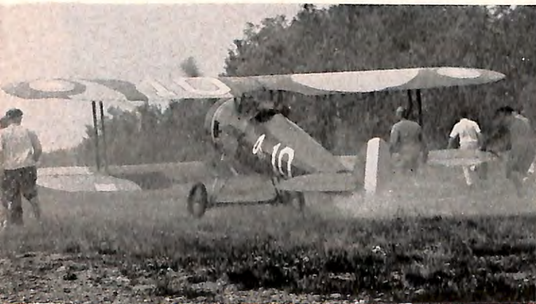
(Above) Since brakes hadn't been invented back in 1918, a ground crew must hold the plane until it reaches airspeed.
