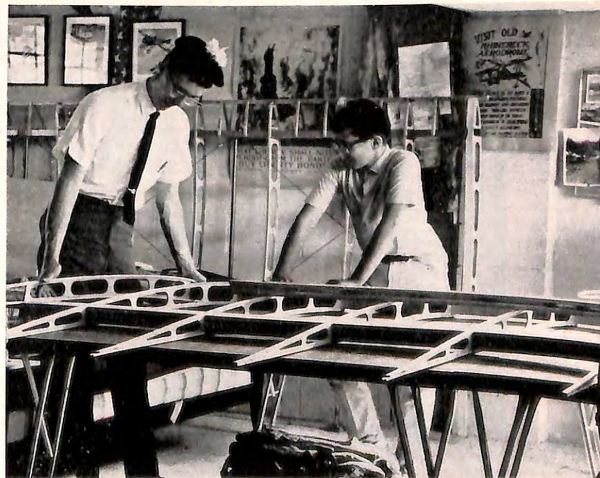
(Right) Pingpong must give way to aviation until Dick King and son assemble a Sopwith Snipe from original blueprints.
