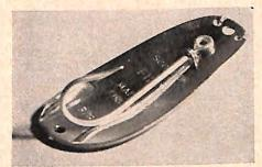
**WEEDLESS LURE** has a spring loaded hook with the tip buried—until a fish strikes. Then it snaps instantly into position, as shown, for hooking the fish before he can spit out the lure.
