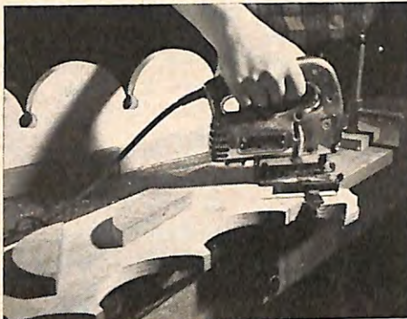
Make a cove-cut edge by swinging a saber saw on a nail driven into a block that is tacked into position against the edge for each circle cut. Scallops in rear were made by first boring 1" holes.
