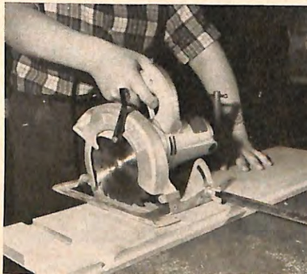
The circular saw can be adjusted to saw to any depth. Here it has formed an edge rabbet (front edge) and is now cutting a second dado across it. A guide is held against work and saw slid along it.
