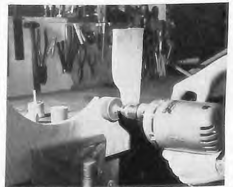
This "driver"-type drill has a speed of 3,200 rpm—enough to do fast sanding with drum (as shown) or with sanding disk. It also has plenty of power for orbital sanding, jigsawing, hedge-trimming.
