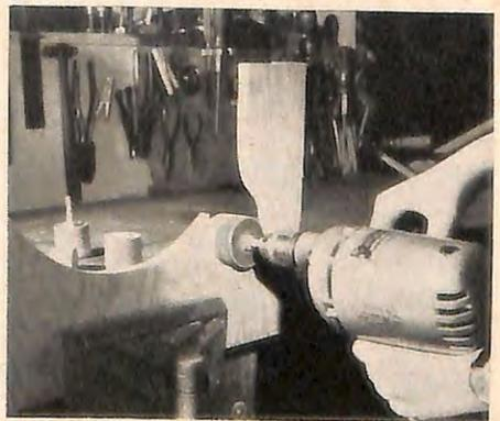
*This "driver"-type drill has a speed of 3,200 rpm—enough to do fast sanding with drum (as shown) or with sanding disk. It also has plenty of power for orbital sanding, jigsawing, hedge-trimming.*
