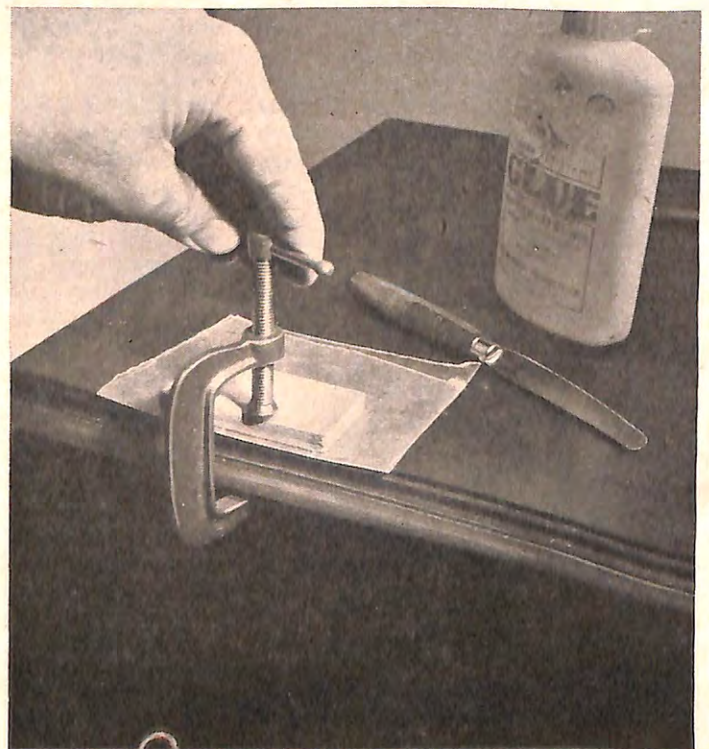
LIFT LOOSE VENEER cautiously to avoid cracking it. Scrape away all the old adhesive. A thin-bladed spatula is useful for applying fresh glue (left, above). Clamp the veneer to the surface firmly, protecting it with wax paper and a wood block, as shown at right.
