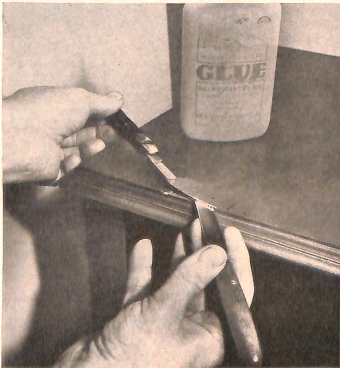
LIFT LOOSE VENEER cautiously to avoid cracking it. Scrape away all the old adhesive. A thin-bladed spatula is useful for applying fresh glue (left, above). Clamp the veneer to the surface firmly, protecting it with wax paper and a wood block, as shown at right.
