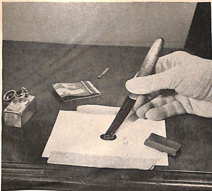
USE A CLEAN FLAME to heat the spatula or knife when applying stick shellac to a gouge or hole. Mask the unmarred surface with paper, and press shellac into the cavity (above, left); holding spatula horizontally (right), build up layers slightly higher than surface.
