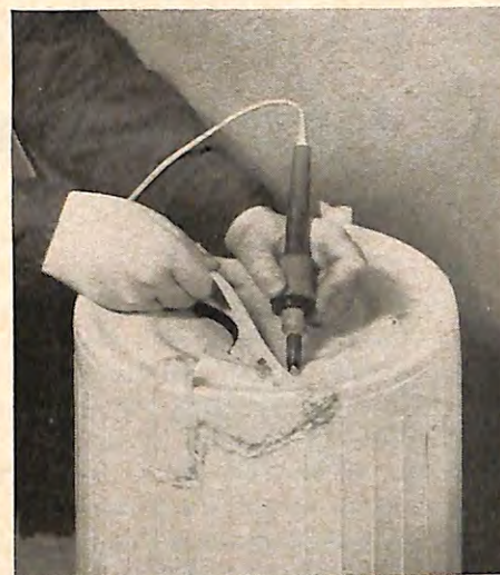
Wastebasket was torn apart when water froze in it outdoors. Material from its rim was fused across the break. Although patch shows, it is waterproof and strong.
