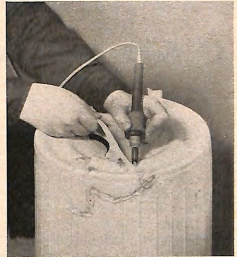
Wastebasket was torn apart when water froze in it outdoors. Material from its rim was fused across the break. Although patch shows, it is waterproof and strong.
