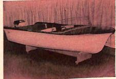
SEA MATE. Made of fiberglass, the Sea Mate (by Tomahawk Boat Mfg. Corp. in Tomahawk, Wisc.) has a "lap-step" de-sign of wide, molded laps. This seamless boat has an 80-inch beam, 40-inch depth, can carry 80-horsepower outboard.
