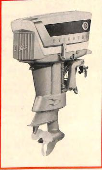
LARK. Refinements on this year's 35-h.p. Lark from Evinrude Motors, Milwaukee, include a soundproof chamber from hood to propeller, a silencer sealed over the exhaust tube, thermostatic water-system control, and fuel saving throttle linkage.
