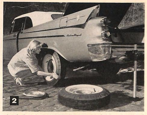
Lay the flat aside, stand the spare up with the hub-cap side toward you, and lift it onto the bolts (Figure 2). These won't line up with the holes in the wheel at first try.
