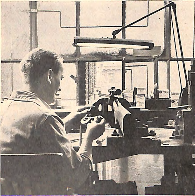
The gunsmith at Stoeger's Long Island City offices mounts a sight with the help of a small target outside the window.
