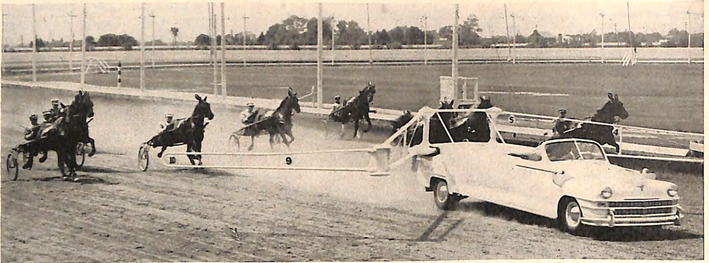
Here is the device that helped bring the trotters back—the Phillips starting gate. The gate, consisting of a pair of folding wings 70 feet in width, is attached to the chassis of a convertible. Car and horses move slowly down the track until the
