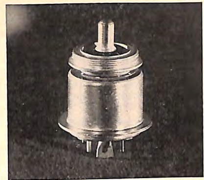
The magical "416-A" vacuum tube, new amplifier which makes possible many of the modern improvements in transmission of telephone, television and radio messages. Created by Bell Laboratories, it is manufactured at the Allentown Electronics Plant of Western Electric.
