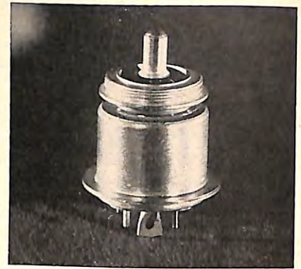
The magical "416-A" vacuum tube, new amplifier which makes possible many of the modern improvements in transmission of telephone, television and radio messages. Created by Bell Laboratories, it is manufactured at the Allentown Electronics Plant of Western Electric.
