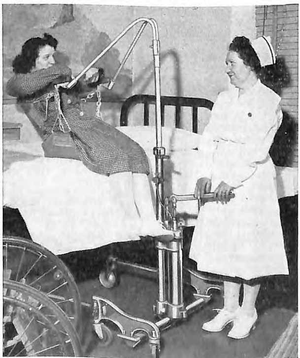
Here is shown the Porto-Lift adapted to transferring a patient from bed to wheel chair. The double arms are used, with the two wide straps, plus the sponge rubber crutch pads. This problem of transfer is done with a minimum of movement for the patient, causing less discomfort, and makes the task for the nurse a simple one.
