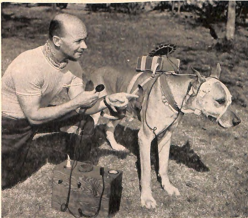
Carl Spitz demonstrates a radio for transmitting instructions by remote control to dogs.
