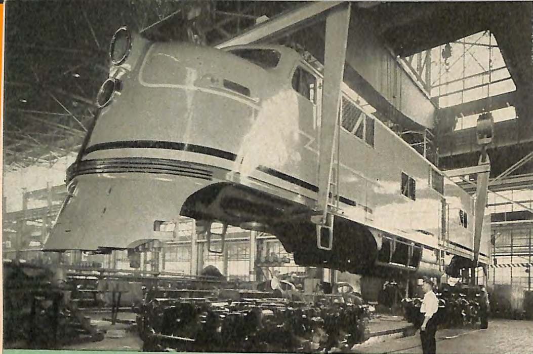
A unit of a 4,000-horsepower Diesel locomotive which will release five steam locomotives for war transportation.
