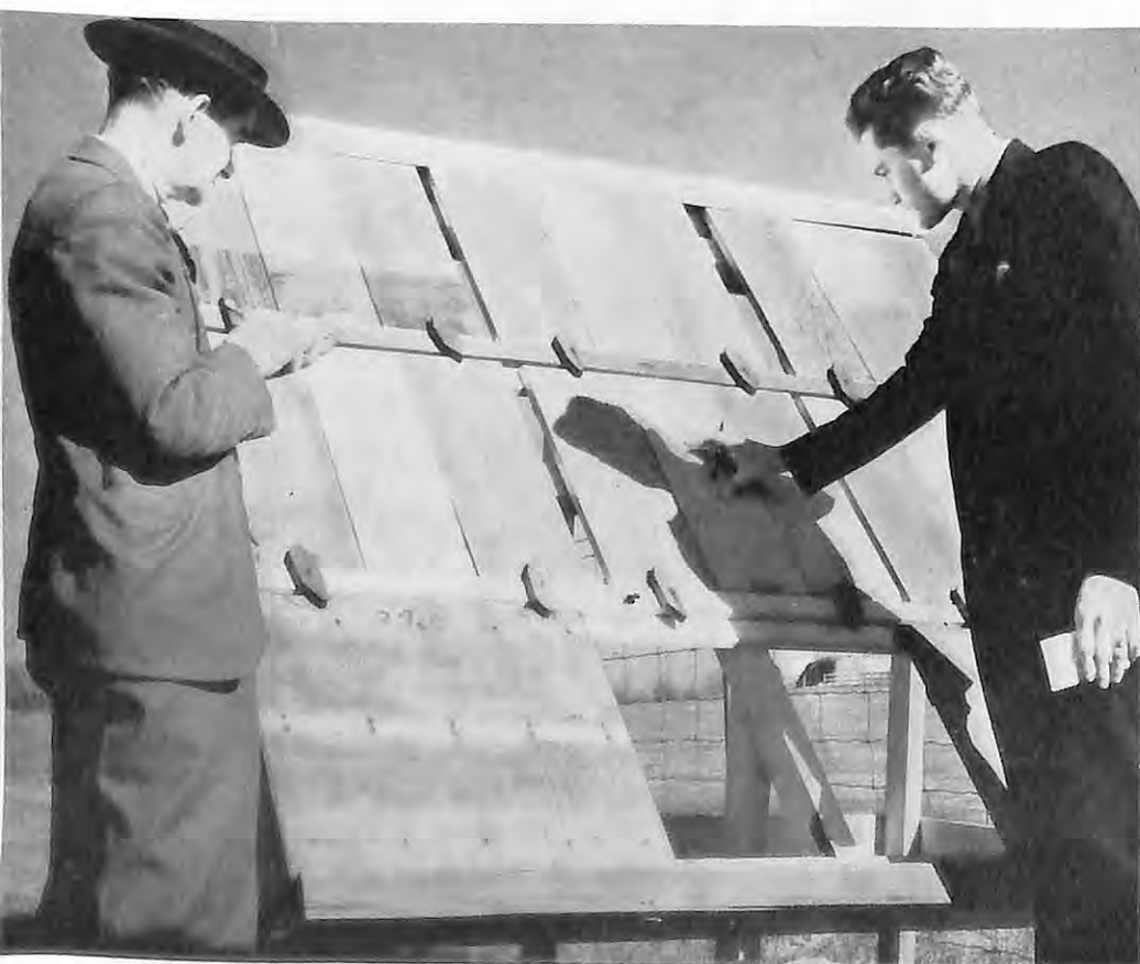
These men are testing the finish of a soybean oil varnish on an exposure rack.
