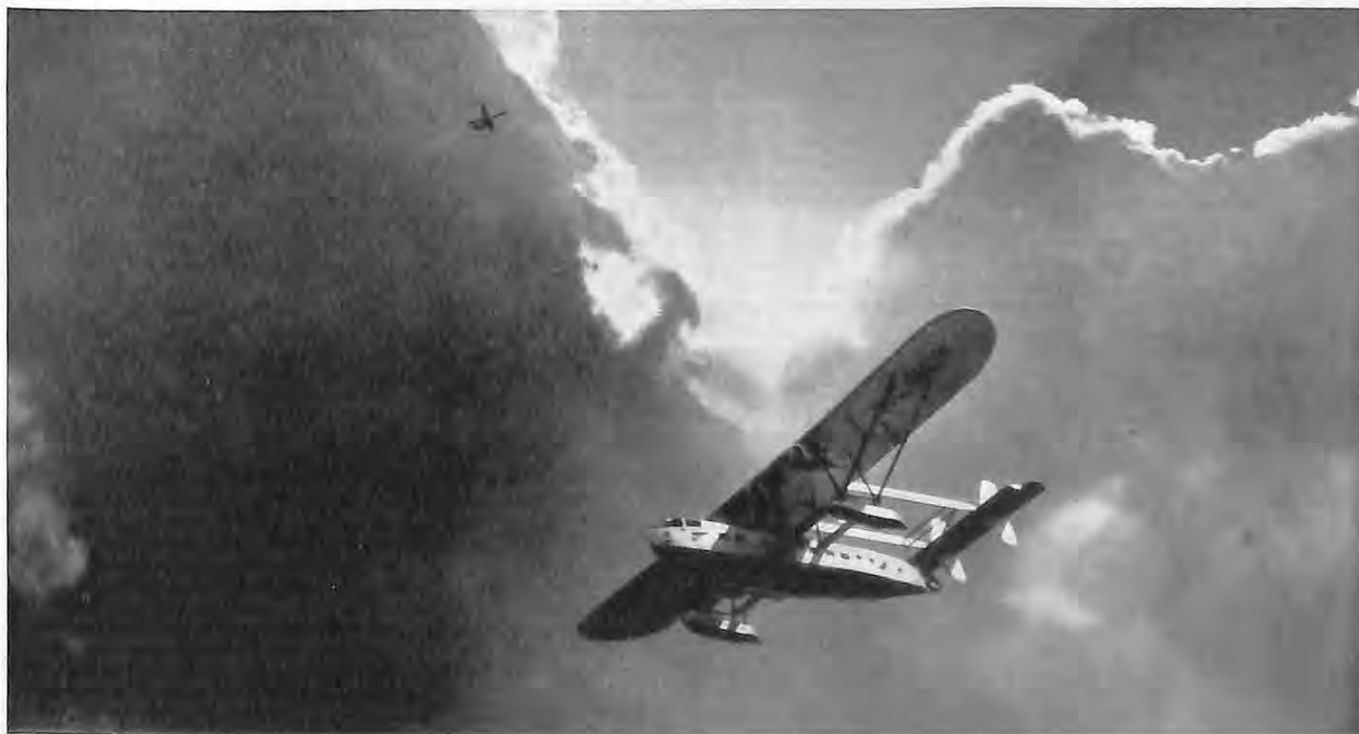
The "American Clipper," largest air liner in service. It carries 48 passengers, weighs 17 tons and its 4 motors develop 2,300 h. p. It was christened in Washington by Mrs. Herbert Hoover and piloted on its first flight to South America by Colonel Charles A. Lindbergh
